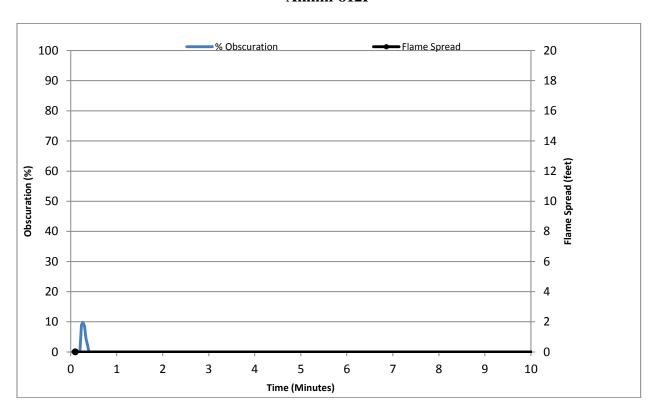
Test Num.: 1 R38267 / 4786842089 06051510 Flame Spread Index: 0 Smoke Developed Index: 0 Max. Flame Spread (ft.): 0.0
