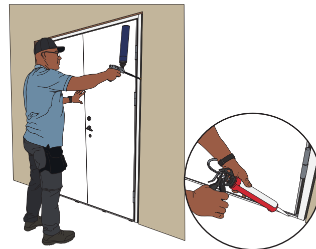
STEP 12. The gaps between the wall and the jamb are sealed with the fire resistant polyurethane foam "Penosil Premium Fire Rated B1" or with the fire resistant mineral wool class A1 or A2-s1, d0.
